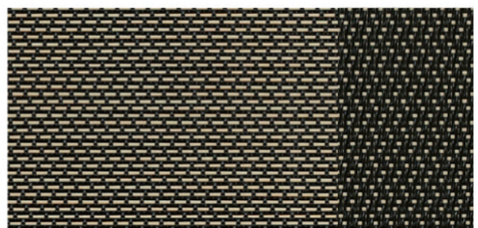
BROKEN TWILL CONSTRUCTION
